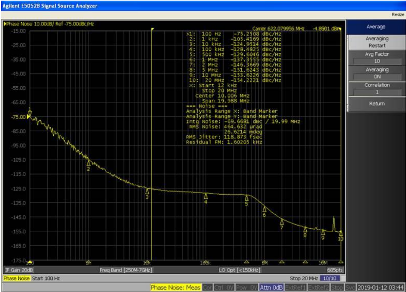
Figure 3. Representative Phase Noise Measurement: F_{OUT} = 622.08\text{ MHz} , F_{IN} = 10\text{ MHz} ,
