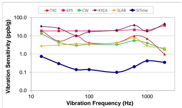
Figure 5. Vibration Robustness<sup>[5]</sup>
