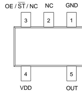
**Figure 1. Pin Assignments**
