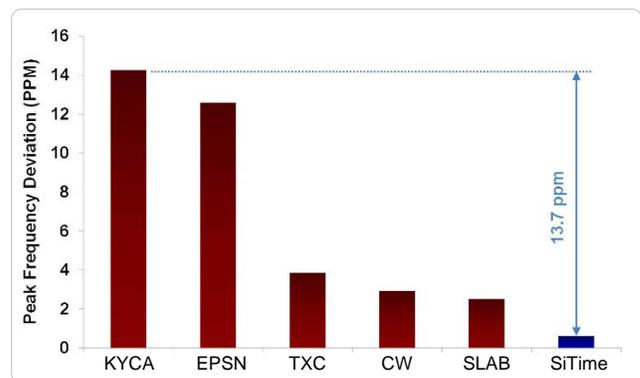
Figure 6. Shock Robustness<sup>[6]</sup>
