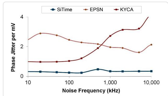
Figure 4. Power Supply Noise Rejection<sup>[4]</sup>
