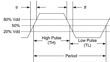
**Figure 3. Output Waveform<sup>[6]</sup>**
