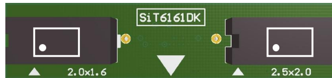
Figure 3. Time Machine socket card SiT6161DK. Supports 2.0 mm x 1.6 mm (4-pin) and 2.5 mm x 2.0 mm (4-pin) packages.
