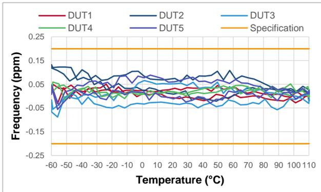
Figure 3. Frequency Stability vs. Temperature
