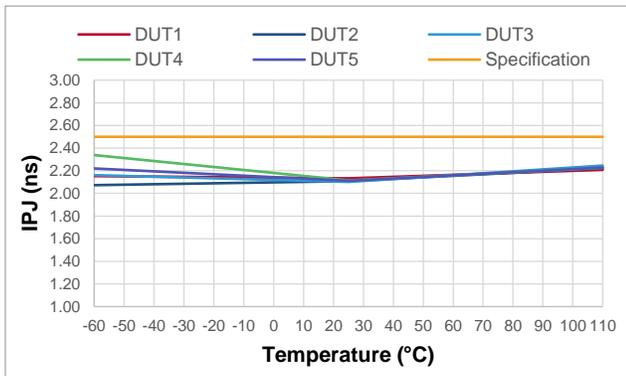
Figure 5. Integrated Phase Jitter vs. Temperature
