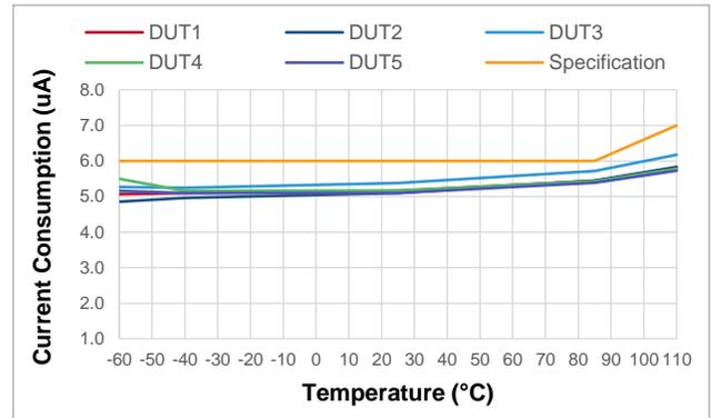
Figure 4. Supply Current vs. Temperature
