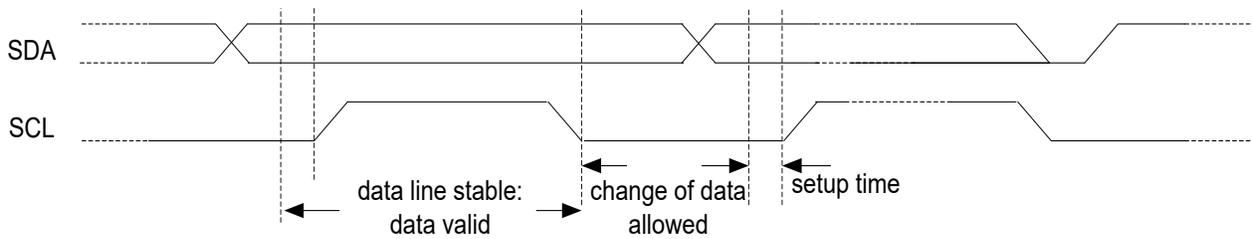
**Figure 42. Data and clock timing relation in I<sup>2</sup>C bus**
