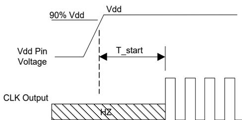
$T_{\text{start}}$ : Time to start from power-off
