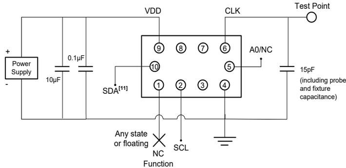
**Figure 12. LVCMOS Test Circuit (I<sup>2</sup>C Control), DCTCXO mode for AC and DC Measurements**
