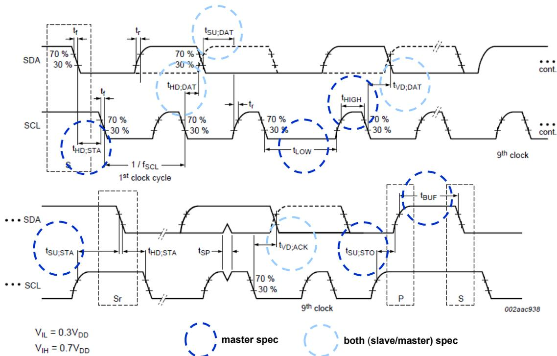
Figure 48. I<sup>2</sup>C Timing Diagram
