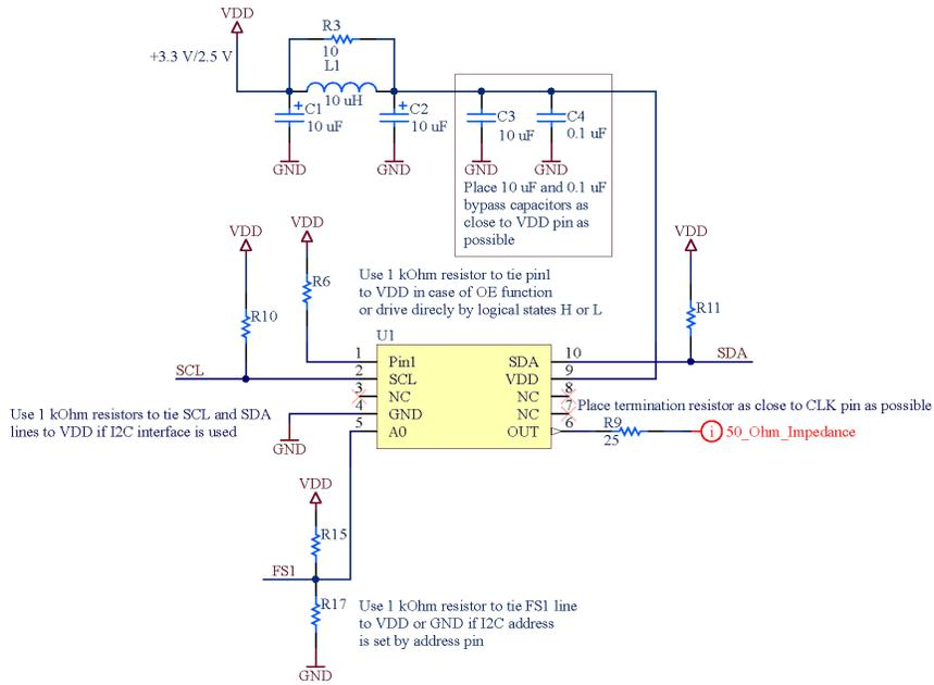
Figure 49. DCTCXO schematic example
