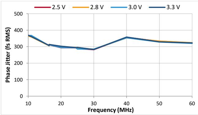
Figure 31. RMS Phase Jitter, DCTCXO, TCXO (Clip Sine)
