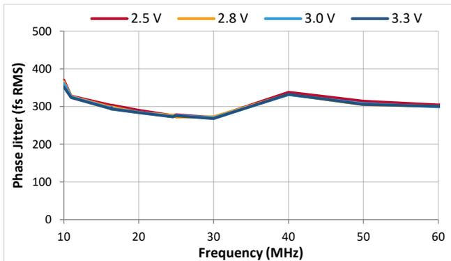
Figure 23. RMS Phase Jitter, DCTCXO, TCXO (LVCMOS)
