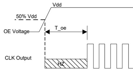
$T_{\text{oe}}$ : Time to re-enable the clock output
