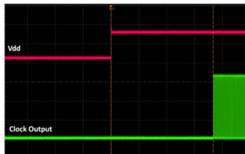
**Figure 16. Startup Waveform vs. Vdd**
