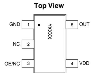
Figure 1. Pin Assignments
