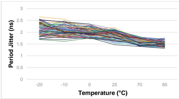
Figure 3. Period Jitter, no supply noise over temperature for VDD = 1.5 V
