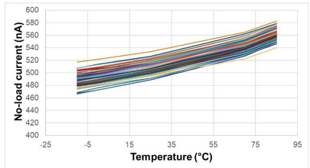
Figure 8. Typical No-load current over temperature for VDD = 1.8 V
