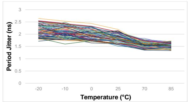
Figure 4. Period Jitter, no supply noise over temperature for VDD = 1.8 V
