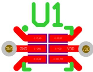
Figure 10. SiT1811 Layout example for board without bypass capacitor
