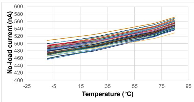
Figure 7. Typical No-load current over temperature for VDD = 1.5 V
