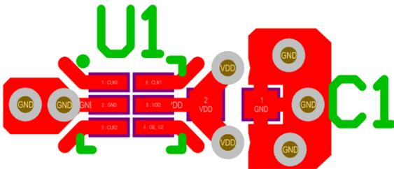
Figure 11. SiT1811 Layout example for board with bypass capacitor
