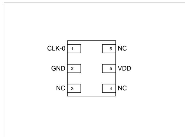
Figure 2. Pin Assignments (Top view)
