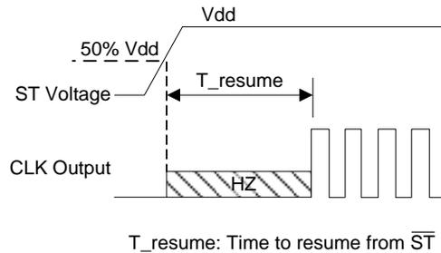
**Figure 5. Standby Resume Timing ( $\overline{ST}$  Mode Only)<sup>[10]</sup>**
