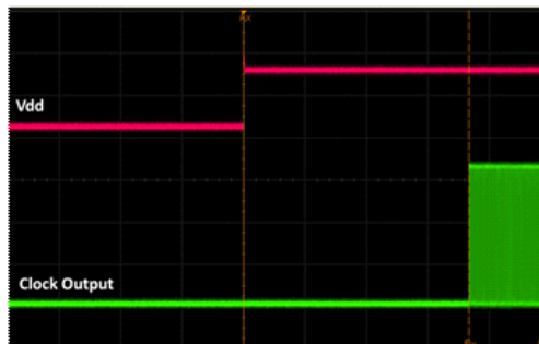
Figure 14. Startup Waveform vs. Vdd
